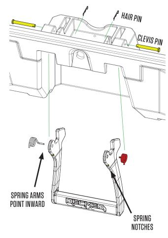
HELPFUL TIP: MAKE SURE SPRINGS HAVE THE LONG ARM HORIZONTAL AND SHORT LEG VERTICAL REFORE INSERTING HANDLE
