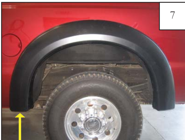
Reinstall bolt removed in Step 1 with a 10 mm socket.
