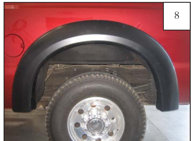
Completed rear flare installation.
