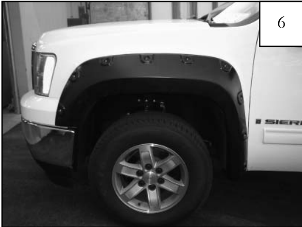
Completed front flare installation.
