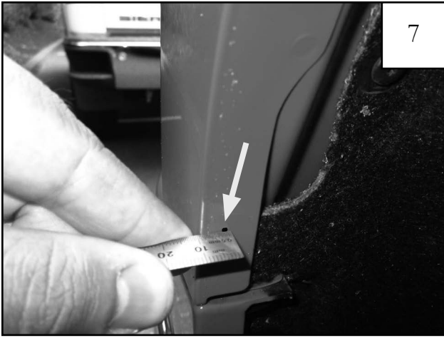
Remove the flare. At the marked location made in Step 5, measure inward 10mm from the edge of the fender. These are the marks to be drilled. Note: Marks at 10mm may be on either side of the first mark.
