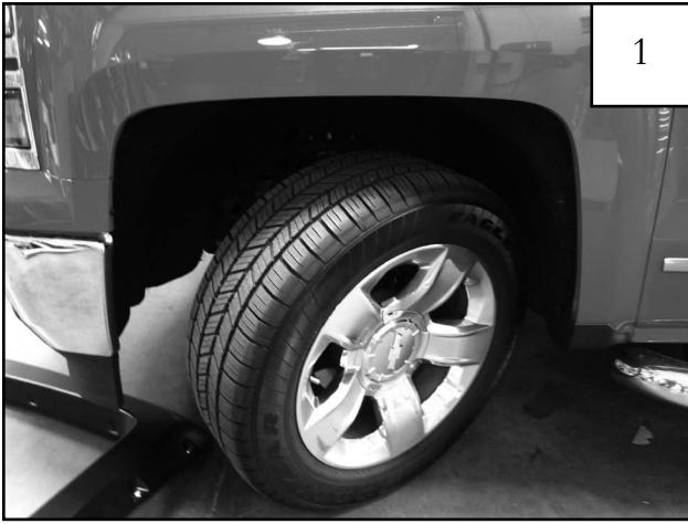
Turn front tire outward for easier installation.
