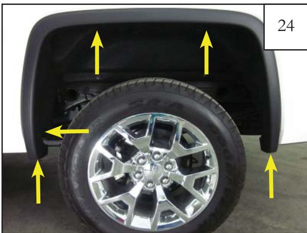
Remove fasteners from factory wheel arch molding using a T-15 Torx Bit for upper and lower wheel well fasteners and a 10mm deep socket and wrench for the lower 2 locations. Save the two lower fasteners for re-installation.
