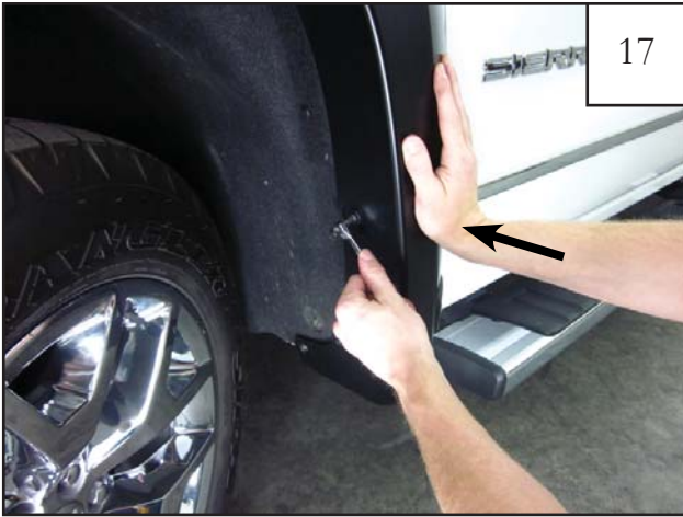
FOR MODELS WITH FACTORY MUDFLAP: Reinstall factory fastener removed from mudflap in step 2. Press flare towards vehicle while fully tightening using a T-30 Torx Bit.
