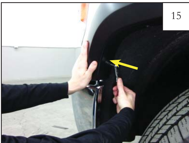
15 While holding Flare on vehicle, install factory screw removed in Step 4 through flare and into factory hole. Do not fully tighten at this time.
