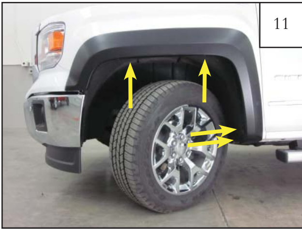
11 While holding Flare on vehicle, install supplied screw (SW1-0056) into the four factory hole locations as shown. Do not fully tighten at this time.
