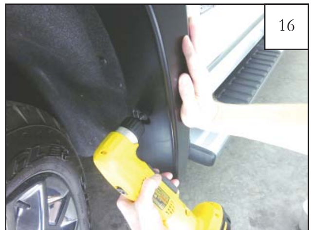
16 Install self-tapping screw (SW1-0066) into pilot hole drilled in step 13. Press flare towards vehicle while fully tightening. Note: This step not needed for models with factory installed mudflaps.
