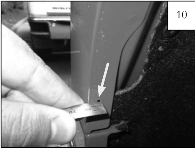
Remove the flare. At the marked location made in Step 8, measure inward 10mm from the edge of the fender. These are the marks to be drilled. Note: Marks at 10mm may be on either side of the first mark.
