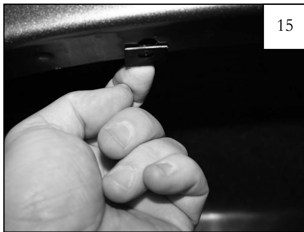
Install Clip (CL1-0022) over existing hole.
