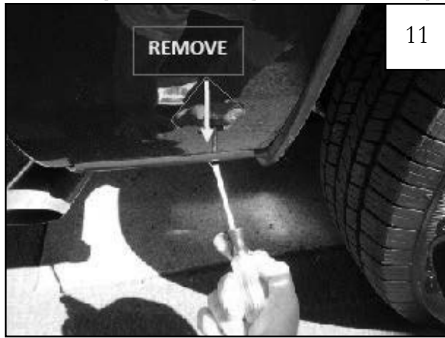
2012 Models Only (Optional): Remove inner piece at bottom rear of wheel well using a pry tool.
