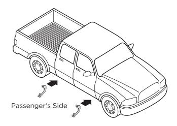
**4.** Align Mounting Brackets with two (2) holes found on the rocker panel (4a) and secure by using two (2) M8 x 30MM Hex Head Bolts, two (2) M8 Lock Washers and two (2) M8 Flat Washers (4b). Repeat this procedure for installation of all Mounting Brackets.
