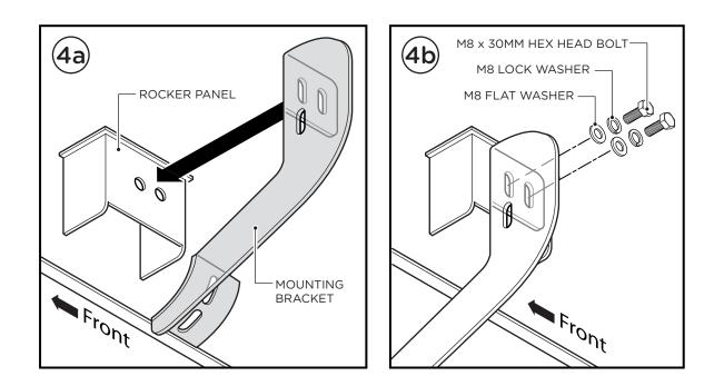
**5.** Align Mount Brace to hole in the rockel panel and fasten using one (1) M8 x 30MM Hex Head Bolt, one (1) M8 Lock Washer and one (1) M8 Flat Washer as shown in (5a) & (5b). Next, fasten the Mount Brace to the Mounting Bracket using one (1) M8 x 30MM Hex Head Bolt, one (1) M8 Lock Washer, (2) M8 Flat Washers and (1) M8 Hex Head Nut as shown in (5c).
