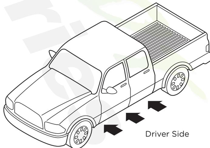
4. Install the Front Bracket using the Front Cab Mount Bolt as shown in diagram.
