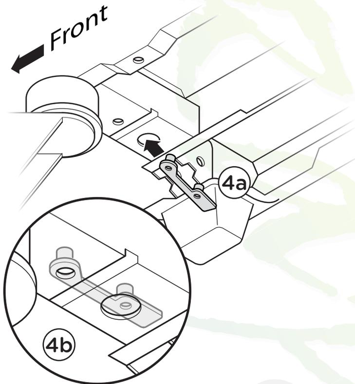
**5.** Align the Front Bracket with the holes on the underside of the vehicle and secure using two (2) M10 x 30MM Hex Head Bolts, two (2) M10 Lock Washers and two (2) M10 Flat Washers.
