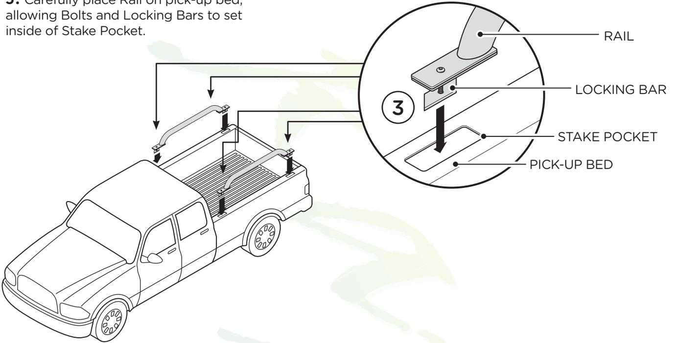
**4.** Slightly lift each end of Bed Rail (4a) and tighten Bolt securely with Allen wrench (4b). As tightening, make sure the Locking Bar catches on both sides of the Stake Pocket Hole (4c).
