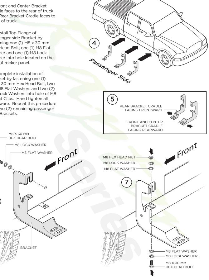
**8.** Place Step Bar and three (3) Rubber Gaskets onto Brackets. Each Step Bar is marked Driver and Passenger.
