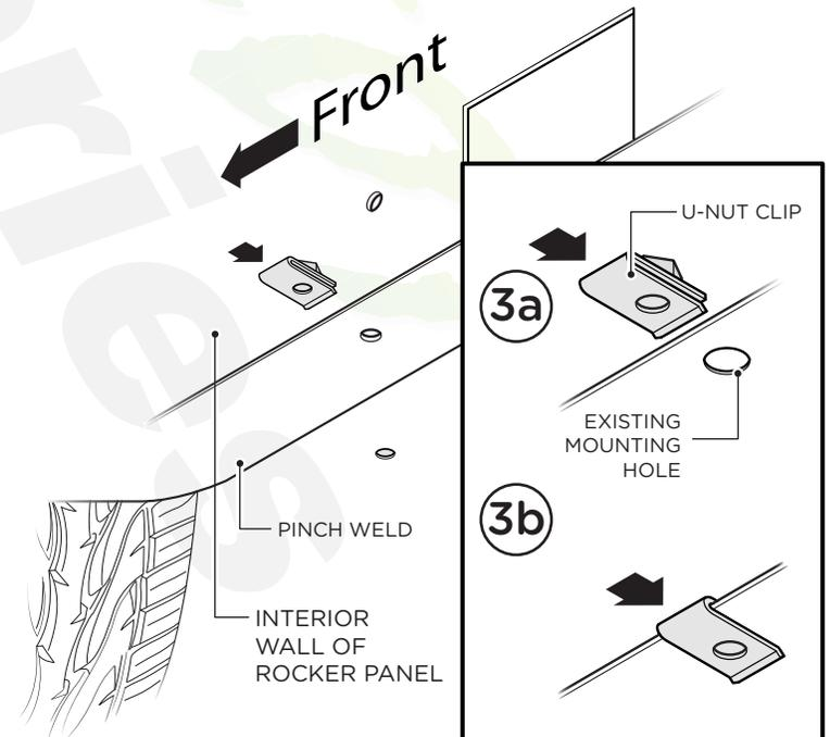
**4.** On passenger side of vehicle, align Front and Rear Brackets as shown.
