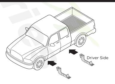
**4.** Insert one (1) M10 Bolt Plate into the hole on the Rocker Panel. Make sure the Plastic Push nut is on the stud of the Bolt Plate to hold it into place.
