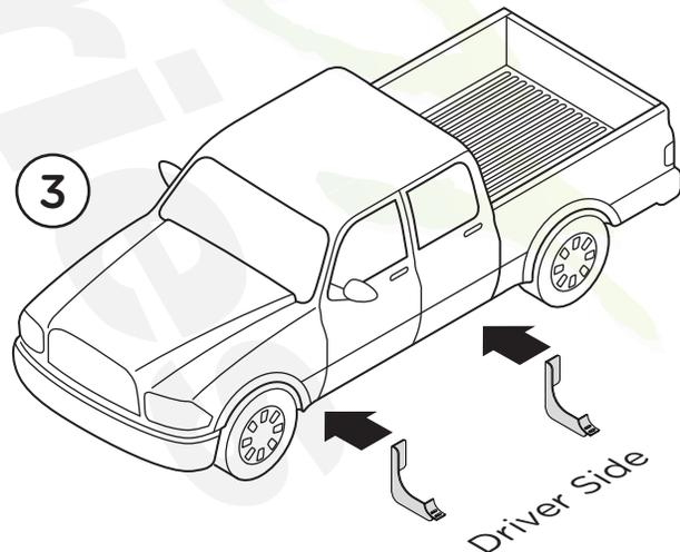
**3.** Install the Plastic Push Nut onto the Bolt Plate shown (3a). Install the Driver Side Bolt Plate into the hole in the frame (3b). The Plastic Push Nut prevents the bolt from falling into the frame and keeps the bolt straight (3c).
