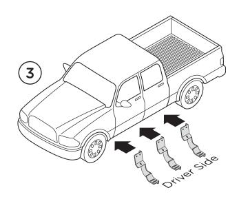
**4.** Align the Front and Rear Driver's Side Brackets with existing bolt and the existing hole located on the Rocker
