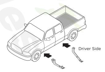
**4.** Install Front Mount Bracket by using one (1) Cab Mount Bolt.
