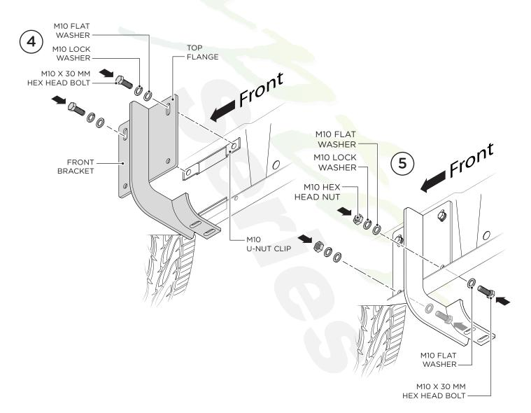
7. Attach the Step Bar to each Bracket using two (2) M10 x 30MM Button Head Bolts, two (2) M10 Lock Washers and two (2) M10 Flat Washers per bracket.
