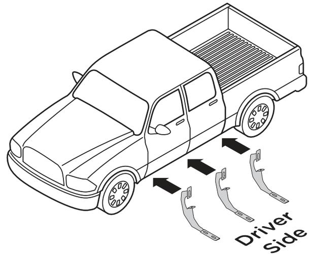
**7.** Complete installation of brackets by placing one (1) Nylon Washer between lower mounting point and pinch weld. Then fasten using one (1) M8 x 30 mm Hex Head Bolt, two (2) M8 Flat Washers, one (1) M8 Lock Washer and one (1) M8 Hex Head Nut. Repeat this procedure for remaining brackets.
